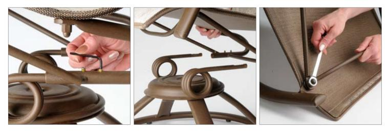
Remove the stretcher bars from the seat basket using the rubber mallet. Be sure to keep note of where the stretcher bars were attached.
